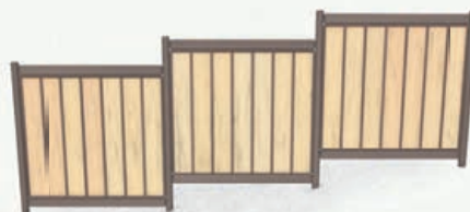
FOLLOWING THE TERRAIN STEPPED
