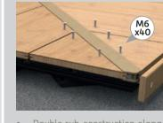
Double sub-construction along the 45° section. Insert sealing tape into the mitre joint on both sides. Only push the composite decking
