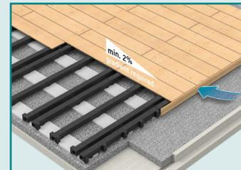
Closed gap with groove strip P5
