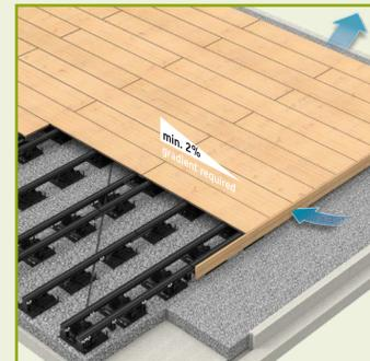
Closed gap with groove strip P5\*
