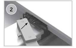
Insert the locked in bracket into the groove in the board.
