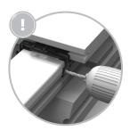
Predrill the construction beam.
