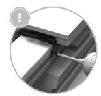
Fix the brackets on the construction beam using the enclosed screws.
