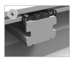
Repeat steps 1 - 4 bis zur letzten Diele. In order to fix the edge of the locking bracket in place, saw a groove (approx. 3 mm wide, 5 mm deep) in the construction beam 10 mm from the edge and position the edge of the locking bracket in place.
