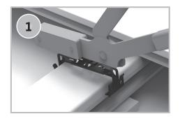
Position the locking bracket on the construction beam using the Zammer (a professional tool comprising both pliers and a hammer) and lock it into place.
