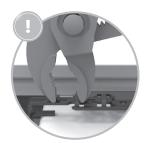
As an alternative, you can also lock it in place using water pump pliers. Place the pliers on the stirrup and hook.
