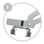
Place the bracket on the zammer before placing it on top of the construction beam.
