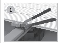
Position the locking bracket on the construction beam using the Zammer (a professional tool comprising both pliers and a hammer) and lock it into place.
