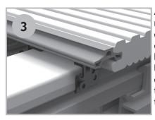
After every metre, fix the clamps to the construction beam in the longitudinal direction of the substructure.
