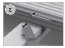
Insert the locked in bracket into the groove in the board.
