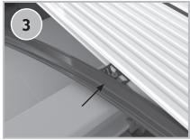
Press the grooved strip from one side to the other, piece by piece, into the groove.
