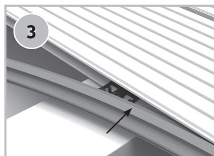
3 Press the grooved strip from one side to the other, piece by piece, into the groove.
