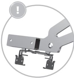
Place the bracket on the zammer before placing it on top of the construction beam.
