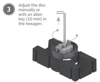
Fine adjustment with engaged construction beam: Rotate the disc manually or by means of a screwdriver. To do this, insert the screwdriver from the side into a discs opening and rotate the disc by lever action. **Tip:** Relieve the load on the construction beam to make it easier to rotate the disc.
