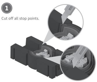
Rotate the rings upwards from the inside to the outside to reach the desired mounting height. Rotate the disc and the rings manually or
