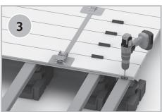
Position the next board. Repeat steps 1&2 for the next 5 boards. Please ensure that the gap pattern is uniform by using a parquet tensioner and megawood® spacers.
