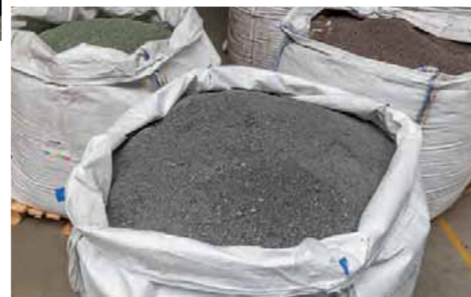
Worn-out decking boards that are returned to us from our take-back dealers are shredded – after separation by type – into a fine granulate. This is returned to the production cycle and used for the manufacture of new boards, which enables us to save valuable resources.
