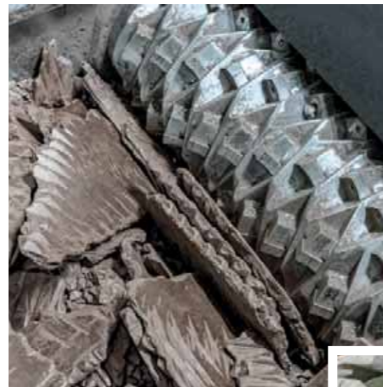
Worn-out decking boards that are returned to us from our take-back dealers are shredded – after separation by type – into a fine granulate. This is returned to the production cycle and used for the manufacture of new boards, which enables us to save valuable resources.
