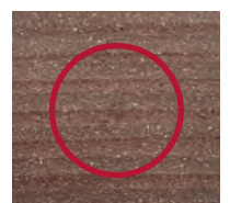
Natural fibre inclusion following mechanical treatment
