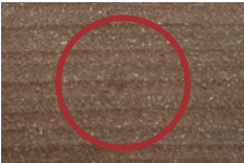
natural fibre entrapment after mechanical treatment
