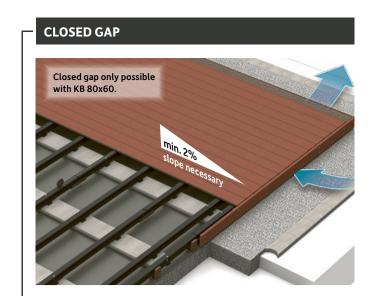
with groove strip / gap profile P5 Only with elevated construction of at least 161 mm, mandatory minimum 2% longitudinal slope of the boards and mandatory sufficient under- and rearventilation (e.g. use of ventilation grilles, rhombus profile spacing).
