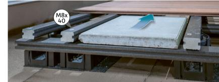
When used for floating construction with VARIO FIX, additional weights such as concrete slabs can be used to secure the deck against wind loads if the deck's own weight is insufficient for the respective wind load zone.
